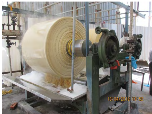
Caption: Cotton dyeing using jigger machine
